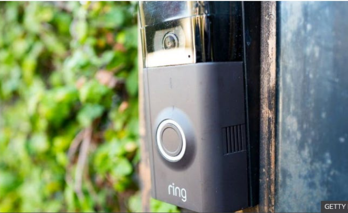
The video doorbells use a screw to keep the faceplate and battery in place.
