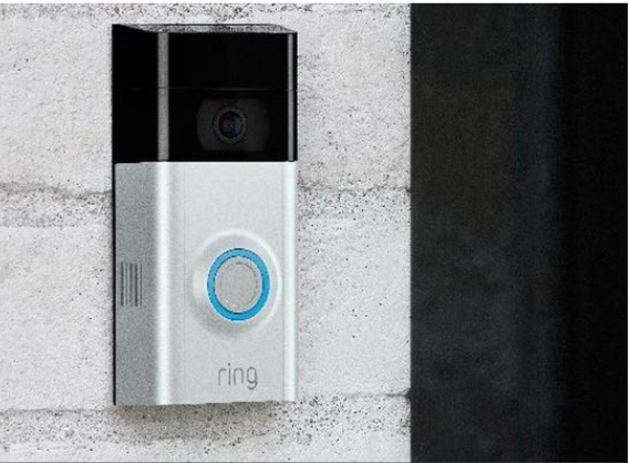
The Ring doorbells use both cameras and motion sensors to detect when someone approaches.
